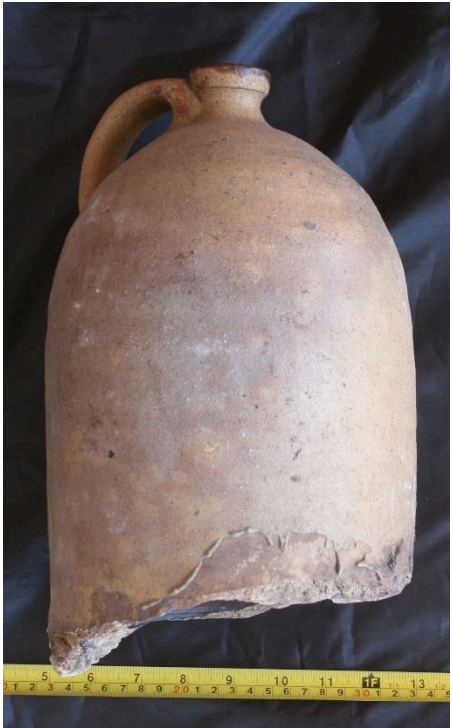
Figure 22: Landrum-Stork jug waster donated by a neighborhood resident. Note the clay condition at the base and the failure of the glaze to mature.
